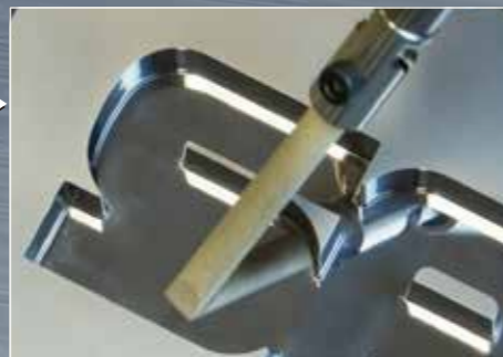
[Finishing] Using wood tip and diamond paste
