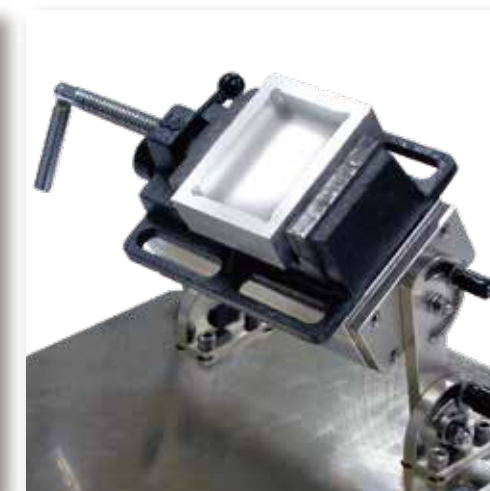
The aluminum mold can be fixed together with the vice.
