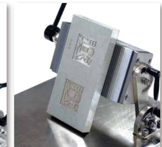
A large-sized mold can be fixed robustly at the desired angle.
