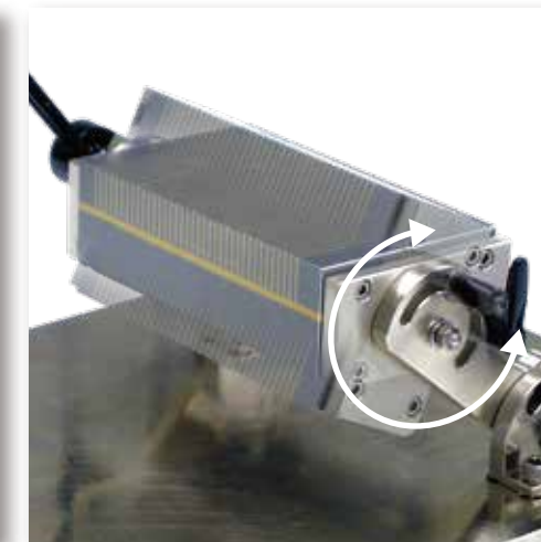
The magnet itself can also be rotated flexibly.
